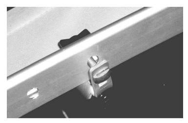
19. When all washboards are in place, engage the T-bolts into the crossframes brackets by pushing them through the slots and turning them 90 degrees so they don't pull back through (see photo at left). You may find it helpful to unscrew the black knobs a little, but don't remove them completely—and don't tighten the black knobs all the way just yet.
