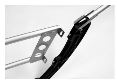
3. Fold the deck strut back so it is out of the way. Locate the two side frames marked *right bow* and *left bow*. Beginning with one side frame, engage the metal keyhole bracket onto the two screws mounted in the keel end (see photo at left). Do not tighten these screws! Repeat with the other side.
